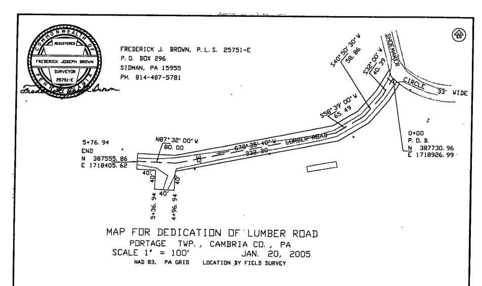
LUMBER ROAD IS 33' WIDE, 16.5 FEET ON EITHER SIDE OF THE ABOVE DESCRIBED CENTERLINE WITH A 40' WIDE TURNAROUND AS SHOWN
